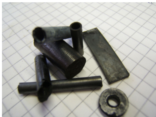
Fig. 9. Emulsion-processed polymer-derived SiC bodies with porosities of 10–35%.
